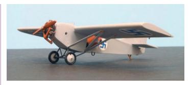
Landing gear struts and the tail skid were built from plastic rod, wing struts from strips of plastic. Some rigging was done using stretched sprue. Windshields were cut from a clear sheet, and the passenger compartment door from .010 inch plastic sheet. The kit has round holes in the forward part of the cockpit. These are too large, and based on looking at the real aircraft, they were not windows.
